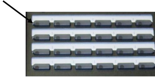
THESE ARE THE 6, 12, OR 24 DUAL COLOR LED BUTTONS ON YOUR PHONES. ANY BUTTON NOT LABELED CAN BE USED FOR "ONE TOUCH" ACCESS TO DIAL OUTSIDE THE SYSTEM OR PROGRAM A SYSTEM FEATURE SUCH AS "MEMO DIAL, BACKGROUND MUSIC, DND, HEADSET, INTERNAL/EXTERNAL PAGE ZONES, ETC.)
