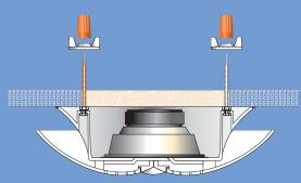
The speaker's two specially-designed studs pierce the ceiling tile.
